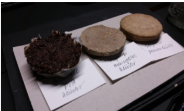
3 samples from the experiment. From left: 1) fomes fomentarius, PVA, natural material based glue; 2) sawdust, ashes, glue; 3) sawdust, glue.
